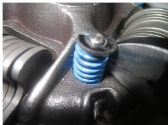
**Step 3:** **FIRMLY** grip side of clip at the **3 o'clock position**
