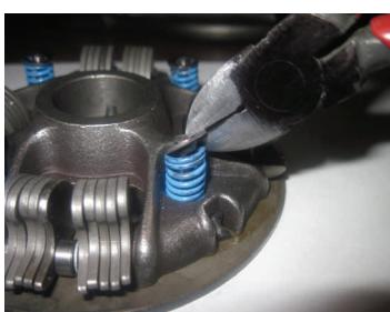
**Step 4:** To reinstall, grip clip **VERY FIRMLY** at the **5 o'clock position**.
