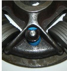
**Step 2:** Push spring sideways away from the **3 o'clock position** (slot is at 12 o'clock)
