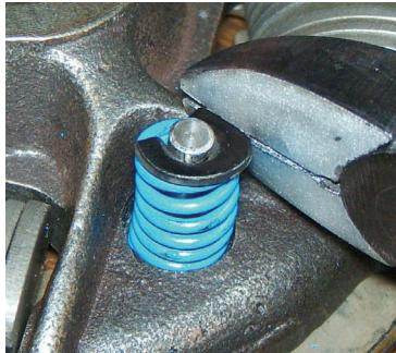
and raise up tool handles in an arc motion and remove clip.
