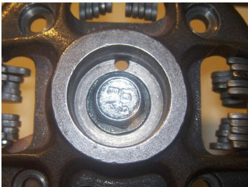
Do not drill through so far as to create a groove on front side.
